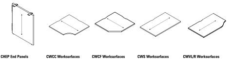
• Communication and electrical wires are routed through a cable scoop located at the back of the Worksurface. When specifying a Straight Worksurface (CWS) or a Curvilinear Worksurface (CWVL), note that the number of cable scoops depends upon the width of the Worksurface. All other Worksurface shapes have one scoop on Panel edges.
